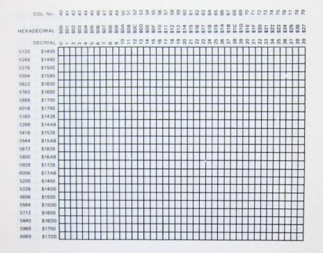
Fig A1.3 80 column text display memory may (right hand side)
