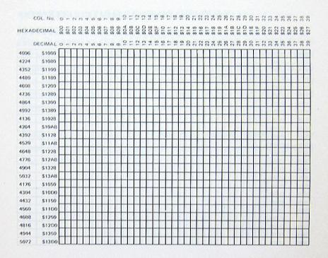
Fig A1.2 80 column text display memory map (left hand side)
