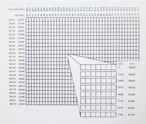
Fig A1.7 Double Resolution graphics display memory (right hand side)
