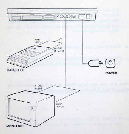
Figure 1.2 Making the wiring connections.
