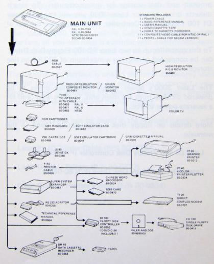
Figure 4.1 Laser 3000 System Diagram
